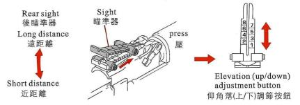
The 031 series rear sight is a tangent type which is adjusted vertically according to distance to the target.
